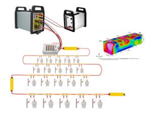
Geomative is the first one in the industry to adopt ERT modules in the high-powered IP mid-gradient cross-sectional profiling. Similar to the ERT method, clients can deploy a pair of AB electrodes and multiple sets of non-polarizable electrodes. AB transmitting electrode is connected to the AB terminal port on the GD-20, while the non-polarizable electrodes are connected to the ERT cables takeouts.
