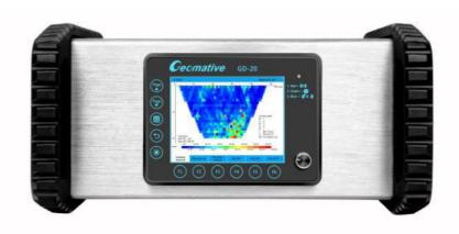
GD-20 is a brand new multi-channel geo-electrical system, designed with 5 and 12 channels. In the process of ERT test, GD-20 can synchronously acquire 10 measuring points which greatly enhances testing speed in the field. It's applicable to Resistivity, Self-potential (SP) and Induced Polarization (IP) test. Compared with single-channel GD-10, the average testing speed of GD-20 ERT system is increased by two to three times and extremely shortens working time.
