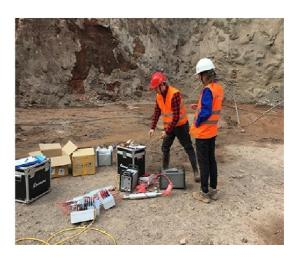
GD-20 is portable and equipped with internal storage for data recording. The multi-channel switch boxes supports VES, ERT and N-∞. VES can simultaneously test 12 sounding points. The ERT test
