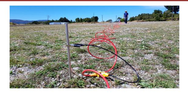
In ERT test, the multi-electrode cable wiring way has the biggest influence on the construction efficiency. The cable volume, weight, wiring efficiency, component reliability, and flexibility to adapt to a variety of environments and needs are very important.
